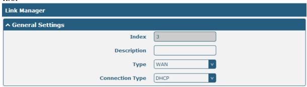
When choose the WAN Connection Type as DHCP, R2000 will obtain IP automatically from DHCP server. When choose the WAN Connection Type as Static.
