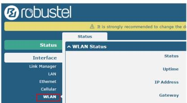
Configure the Wi-Fi AP please go to the **Link Manager > WLAN** tab, and the way of configuration refer to the **3.6 Interface > Link Manager** section.
