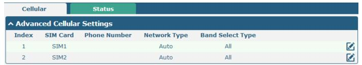
Click ≤ to set the SIM card's parameter according to the application requirement.
